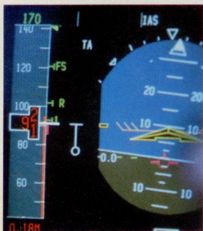
The G-V cockpit has the Honeywell SPZ-8500 avionics suite. Displays include engine information and crew alerting system (EICAS) functions and synoptics pages showing the status of each system. Banks at altitude can be made with confidence, while the "cat's whiskers" warn of lift degradation (below).
