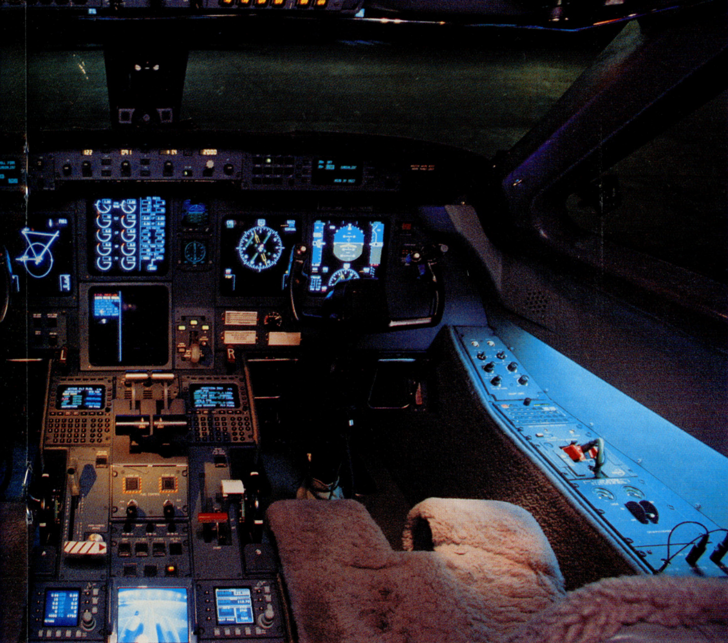
The G-V cockpit has the Honeywell SPZ-8500 avionics suite. Displays include engine information and crew alerting system (EICAS) functions and synoptics pages showing the status of each system. Banks at altitude can be made with confidence, while the "cat's whiskers" warn of lift degradation (below).
